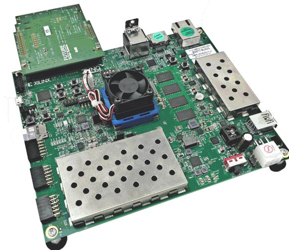
**Figure 1: ZCU104 Evaluation board with CON-FMC**
